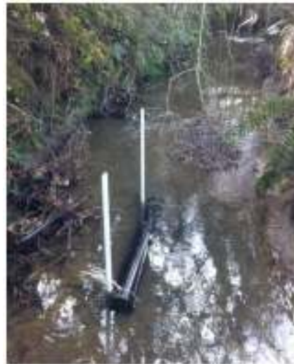
A sediment trap. The water enters a funnel, slowing it down and depositing the sediment
