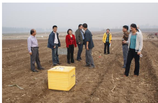
Gas chamber for measurement of direct GHG fluxes ( \text{N}_2\text{O} and methane) from the soil surface, in this case in a maize field on the North China Plain.
