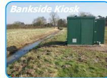
Catchment walkover surveys identify potential **sediment source areas** for sampling. Instream suspended sediments are collected at high-resolution (60 min) during rainfall events by bankside **automatic water samplers**.
