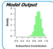
Resulting geochemical data is run through a comprehensive **Bayesian mixing model** to quantitatively apportion the masses of fluvial sediment derived from each source area within realistic levels of uncertainty.
