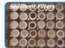
After wet filtering samples, sediment geochemistry is analysed directly from sediment covered filter papers by X-ray fluorescence spectroscopy (**XRFS**) and diffuse reflectance infra-red Fourier transform spectroscopy (**DRIFTS**).
